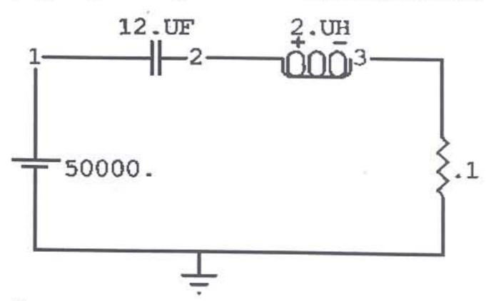
Figure 1. The Basic Representation of the Internal Dynamics. During the initial experiments,  $2\mu$ F were used. During later experiments, the capaitance was increased to  $12\mu$ F. Connections inside and outside of the capacitors have inductance and resistance.
